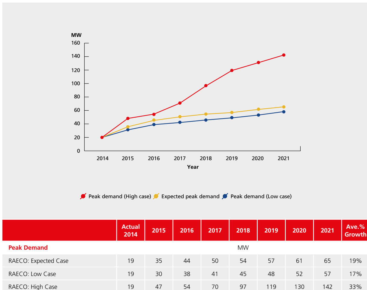
Figure 17 Electricity Demand Projections – Ad Duqm
